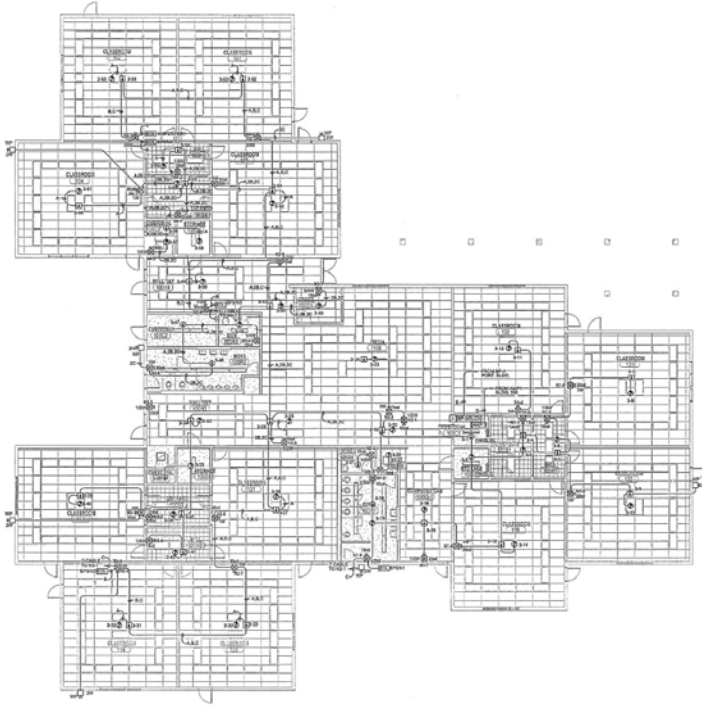
BLDG. 100 FIRE ALARM PLAN SCALE: 1/8" = 1'-0"
